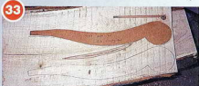
33 When marking out the arms, look for any curves in the grain that follow the shape
