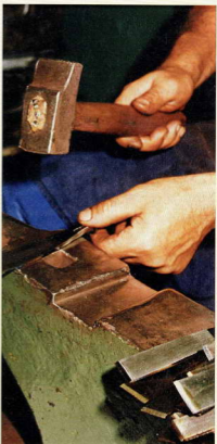
The tool's shape is made perfect by tapping the cold metal while it is still soft, prior to heat treatment
