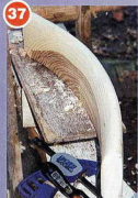
37 The crest rail is bandsawn from a solid section of 3in ash...
