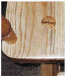
The legs pass through the seat and are wedged across the grain
