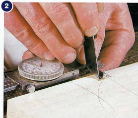
2 The position of each shelf is marked out, together with the width of the trench. This reduces the risk of accidentally cutting the trench on the wrong side of the line
