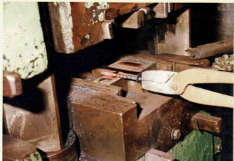
The initial shaping of the red-hot steel is done using a mechanical hammer
