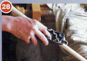
28 ...before a block plane shapes the swelling in the bottom third section
