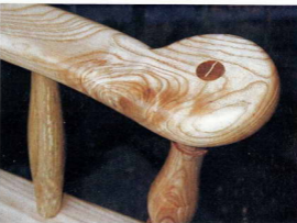
The arm is rounded in for a comfortable feel on the hand. Note the through and wedged joint
