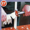
27 The long sticks can be produced using a \frac{3}{8} in rounder, which goes two thirds of the way down...
