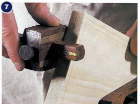
6 The width of the tongue must match the cutter used to cut the trench. It's marked out in the usual fashion
