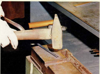
Repeated light hammer blows are used to form the tool's shape. These repeated blows impart characteristics to the steel that cannot be obtained by the single high-energy blow used in the mass-production drop-forging method
