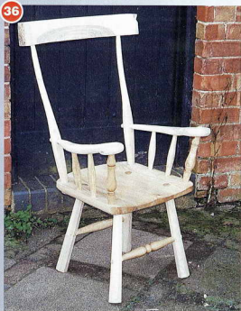
36 The roughed-out crest rail is useful for holding the corner post in situ while the glue sets
