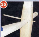
35 The back of the arm passes right through the upright and is also pegged
